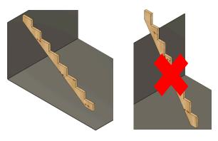
1- place your stringer in the correct direction. The height of each step is 170mm (17cm) The depth of each step is 250mm (25cm)
