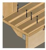
Attention: as you should not allow more than 60cm between the stringers, the steps will pass left and right of the stringer for stairs with a width of 80-100-140-160cm
