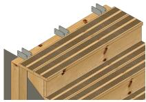
5. Fix the brackets for the top stringers on top of the support with the screws supplied with the brackets.
