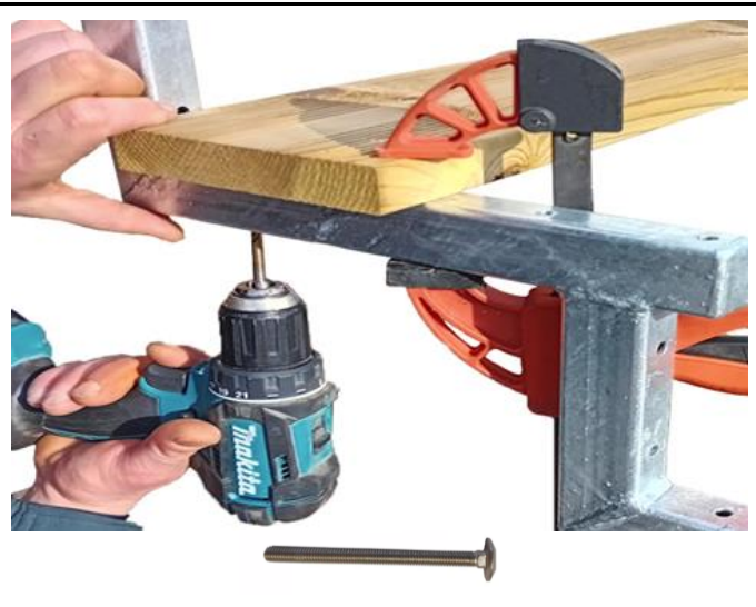
5b - Secure it with clamps and pre-drill the board from below through the stringer's holes and insert the bolts with a hammer (not yet the nuts and bolts).
