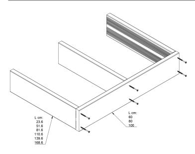
First, create the structure of your step. Each step has 2 different lengths of boards:
