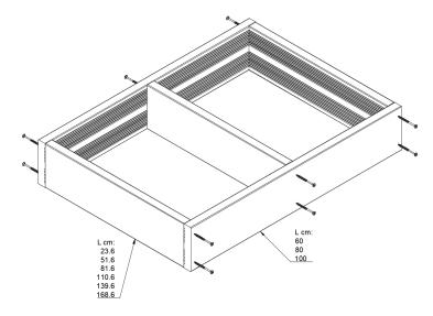
It's recommended to pre-drill the holes with Ø3mm to avoid splitting the wood.
